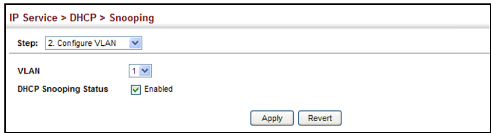
Figure 225: Configuring DHCP Snooping on a VLAN
