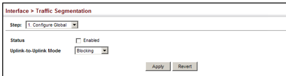
Figure 61: Enabling Traffic Segmentation
